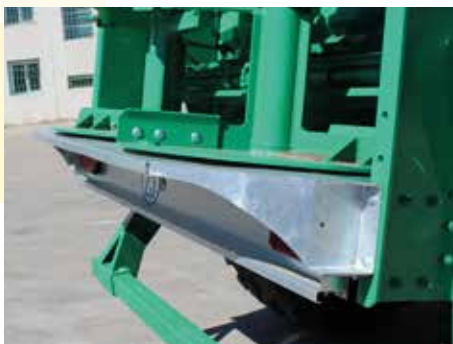
• Bandeja exterior en 2 rulos verticales Outer sheet in 2 vertical auger beaters
