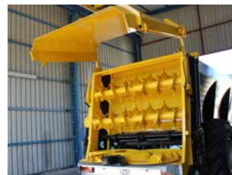
• Compost 2 rulos horizontales + platos (Tritón 95 y Premium 120) Special group for compost of 2 horizontal auger beaters + plates (Tritón 95 and Premium 120)
