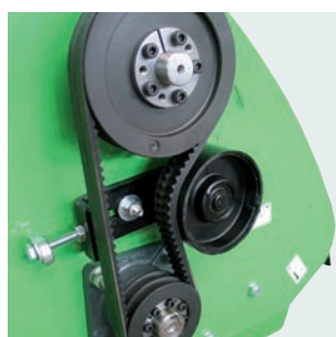
Facile tensione cinghie. Easy belts tightening adjustment.
