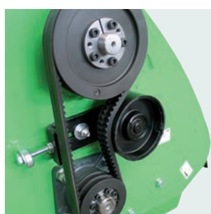
Facile tensione cinghie. Easy belts tightening adjustment.
