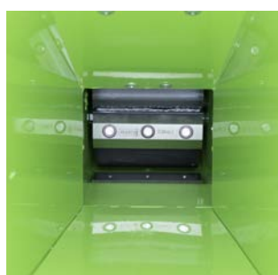
Tamburo cippatore (150 mm x 150 mm). Chipping drum (150 mm x 150 mm).
